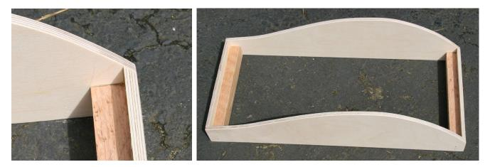
I then attached the <sup>3</sup>/<sub>4</sub> inch square material to the top of both the bow and stern pieces, This would allow for a good square edge for attaching the sides. I attached the sides with glue and clamped the sides along with a two brads in the <sup>3</sup>/<sub>4</sub> inch square material. I placed the hull pieces topside down on a flat surface and checked alignment with a T-square. This gave me a hull that was perfectly square.
