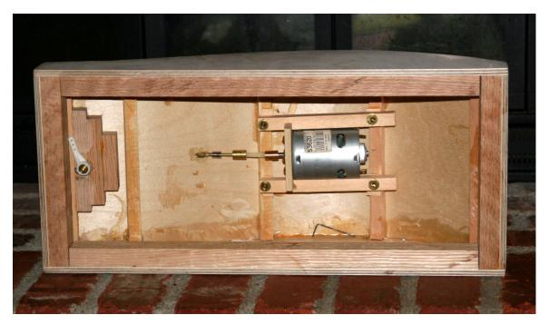
I next fashioned a platform on each side of the motor to mount the batteries. This allows me to mount a  $3\frac{1}{2}$  Ahr 6 volt battery on each side and move it forward and aft to ballast the boat.
