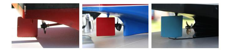
Next I mounted the motor. I fashioned a motor mount that attached to the stringers I had attached to the bottom to assist the bending during gluing. This mounting concept allows me to put in different motors. While I choose an inline arraignment others have used a belt drive that allows the motor to either be placed inline like shown here or with the motor mounted aft over the propeller shaft. Club members have used all three arrangements with good results.
