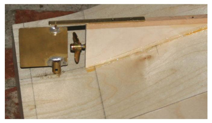
The choice of rudder with or without a skeg is optional except for boats built to play water polo. The pictures below show three variations ranging from no skeg to a skeg and finally a skeg with a shoe under to propeller.
